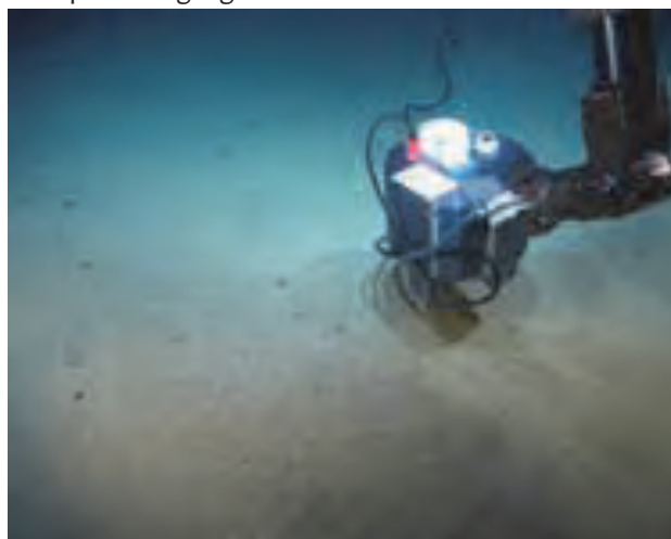
Seismometer connected to the ANTARES secondary junction box (Credit: ANTARES )
