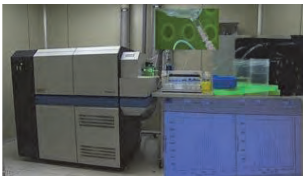
The inductively coupled plasma mass spectrometry (ICP-MS) system. (Credit: INFN)
